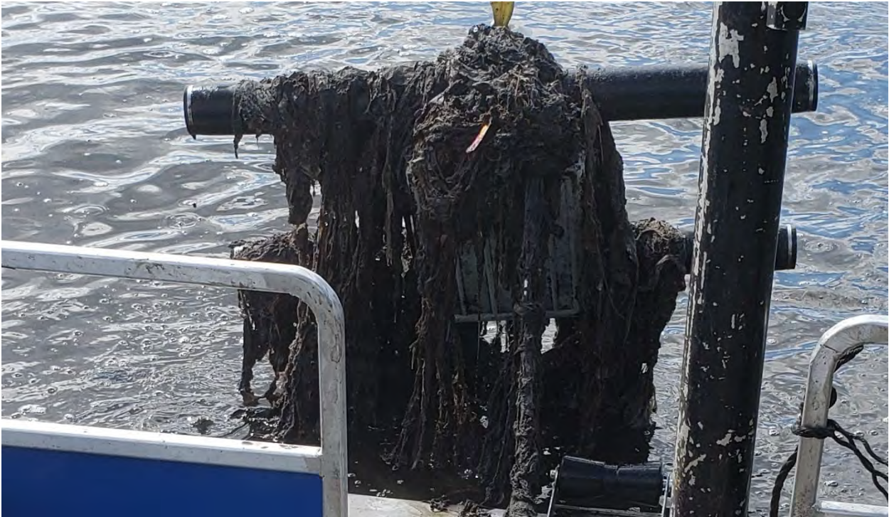
FIGURE 3-6: EXAMPLE OF AN AERATION DIFFUSER FOULED WITH RAG
